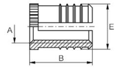
Female thread A = M5 Length B = 10.0 Min distance to edge = 3.0Number of cramping feathers = 5Outer diameter E = 7.00
